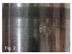
Current passage has led to a formation of craters/flutes on the inner ring raceway (fig. 1) and the lateral surface of the rolling elements (fig. 2) of a cylindrical roller bearing
